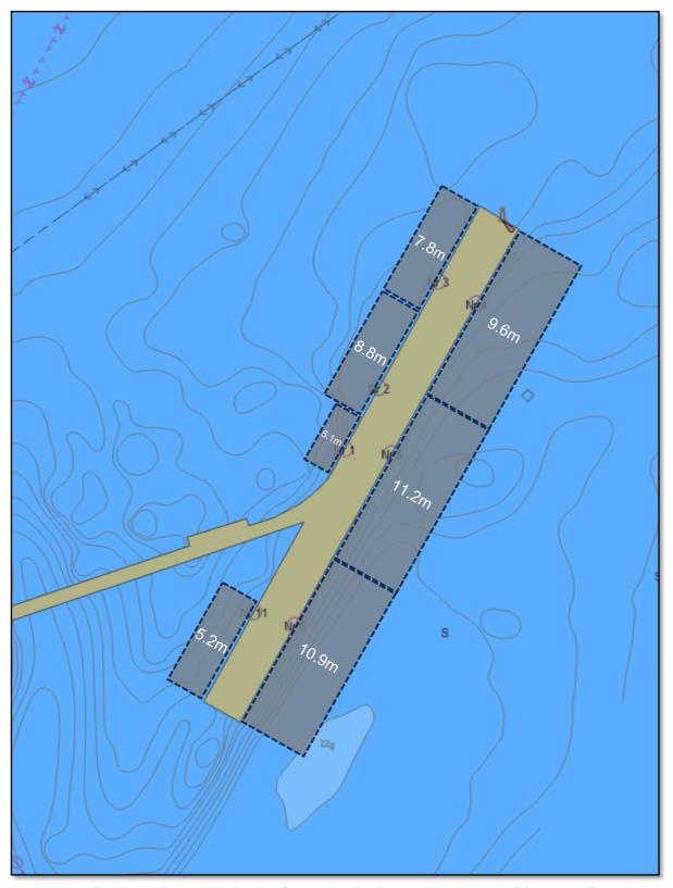
Berth pockets with depths (based on hydrographic survey of Aug 2024)
