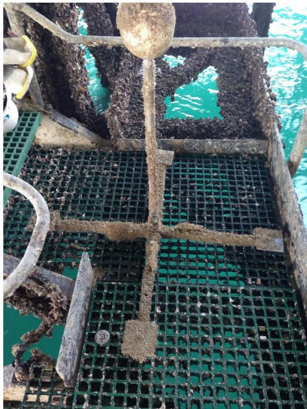
*Array from State Wide Array Surveillance program (SWASP) after two month soaking period under wharf*
