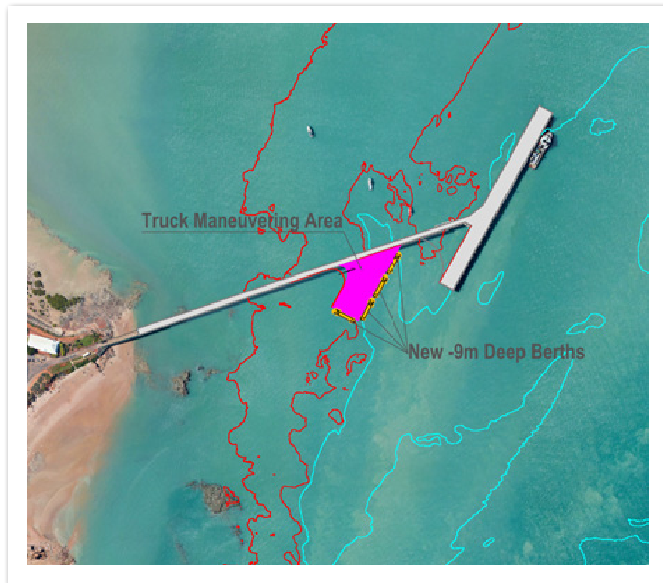
Figure 13 Option 3 - Berths on the Southside of the Wharf Access Jetty
