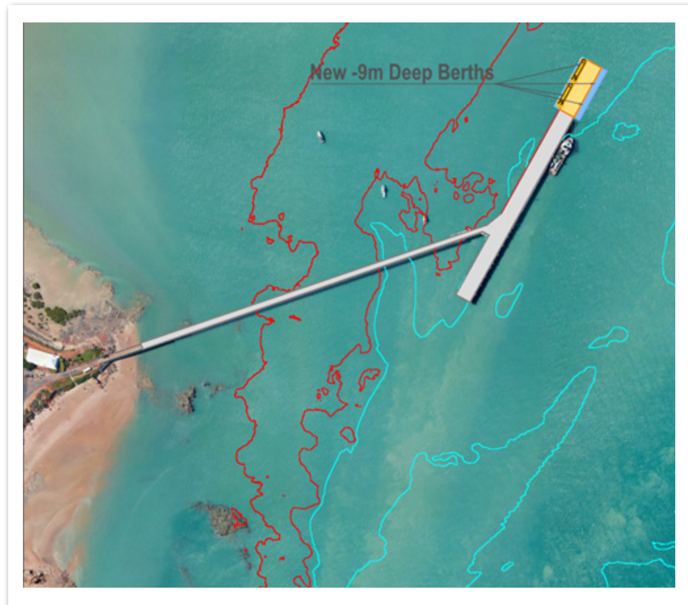
Figure 11 Option 1 - Expansion of the Existing Wharf Toward North
